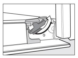
Release the locking clamps by turning them as far as they will go. Do not attempt to take the door off the retainers when it is in the horizontal position as the retainers will spring back against the oven.
